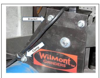
Photo 2 – Mounted Lamp & cable Clamp
