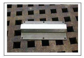
Start by attaching the baseplate and the aluminum solid bar as in photo 1 using 5ea ¼-20 x 5/8 flat head bolts, Machine shop messed up one hole location. I put a setscrew in that hole (Dont use) If you have newer plated LB go to middle of second page now.
