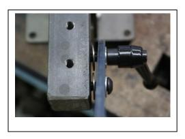
Place large diameter 3/8 washers which are called fender washers between the flat platen and the flat platen arm.
