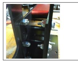
Put the left upright vertical on next using 1" long ¼-20 hex bolts. Ensure you **do not** have washers on the inside under the nut.
