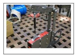
Next attach the threaded eye pieces to the gas shock and then mount the gas shock as in the photo. Ensure the small diameter sliding part of the gas shock is facing down.
