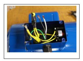
You can see in this photo the waterproof gland was placed in the hole that was created earlier and a 120V cable with a black/white/green wire was introduced into and through the wire clamp. Next tighten the nut on the outside to clamp onto the wire. Next remove the screw on the inside of this enclosure and attach the green wire coming from the power wire through it and tighten it back down.
