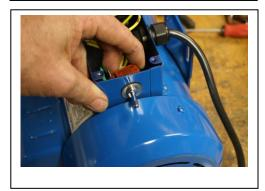
Next place another larger ½ washer on the outside of the switch after it has been placed through the hole from the inside, and then thread on the waterproof boot. The waterproof boot consists of a boot and a nut. The boot must be placed over the nut to create a waterproof/dustproof seal.
