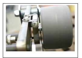
Using a ½-13x3" bolt emplace three washers under the head of the bolt and **two** between the tracking wheel and tracking wheel plate. Tighten the bolt.
