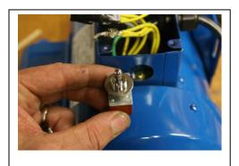
Next knockout the knockout at the end of the electrical box for your power switch. Remove the round nut and washer that is currently on the switch and dispose of them, and ensure the hex shaped nut is threaded all the way down on the bottom of the shaft. Next place the included smaller diameter ½ washer on as pictured.
