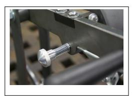
Next thread in the tracking knob with a spring and Washer between the spring and body of the grinder.
