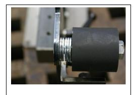
Using a 3/8-16 x 3" bolts place 6 washers between the 2" wheels and the flat platen. Do this on both 2" wheels.
