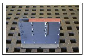
Place the left panel on and the two nut plates that house the 3/8 nuts. Place the two 3/8 nuts in the hex pockets as in the photo.
