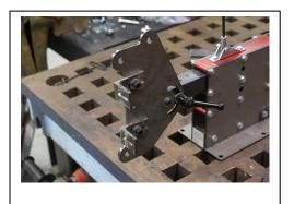
Next attach the flat platen to the arm using the provided 3/8 button head bolt and the  $3/8-16 \times \frac{3}{4}$ " adjustable handle. Ensure you place a 3/8 washer between the bolts and the flat platen. Also attach the angle to the flat platen using  $1/2-13 \times 5/8$  Allen headed bolts with a washer.
