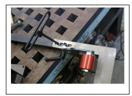
Lastly attach the toolrest to the bottom of the flat platen arm using  $3/8-16 \times 3/4$  allen headed socket bolts
