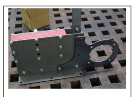
Now undo the bottom two rear screws and attach the motor mount plate. Next attach the other vertical upright on the outside of the motor mount plate
