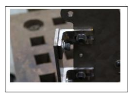
Ensure you place 1ea 3/8 washers on the bolt going through the angle brackets holding on the flat platen plate.
