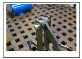
Next using a 3 1/4 " long bolt and two nylon spacers attach the upper pivoting arm as in the photo. Tighten the nyloc nut until the pivoting arm will not swing freely and slowly loosen until it just moves freely.
