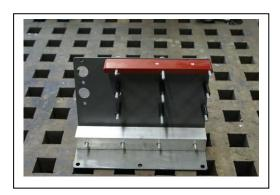
Just about ready for the left panel. Notice the Top red spacer has the threaded holes for the gas shock
