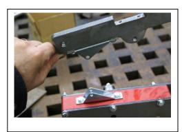
Next attach the two gas shock mounts as in the photo using the  $\frac{1}{2}$ -20 x  $\frac{1}{2}$ " long hex bolts and washers.
