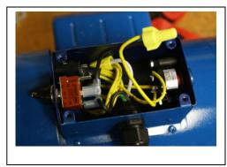
Next take the black wire coming from the 120 cord and place it on the bottom of the switch. Using the included short black wire attach it to the middle position of the switch and then to the T1,T3 and T5 wires using a wire nut included.
