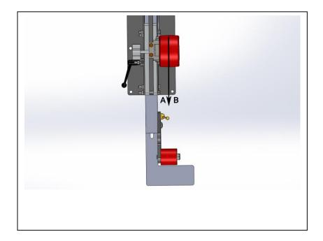
If your tracking wheel is pointed more towards **A** as in the photo above your sanding belt will want to go left and into the body of the grinder. If your grinding wheel is pointed more towards **B** then it will favor the right and want to run off of the grinder. If you can not easily track the belt ¼ off the right and left side of the flat platen plate then it is favoring one side or the other.
