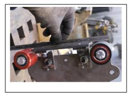
Ensure the flat platen plate is on the same plane as the wheels. I am using a rule to ensure they are all lined up. If not adjust the flat platen plate in or out. Do this also on the ends of the 2" wheels to ensure the 2" wide plate is centered on the wheels
