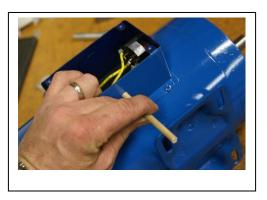
All wiring in the next several steps is done with power cord <u>UNPLUGGED</u> Next remove the electrical box cover from the motor, and pop out the center bottom cutout for the Electrical wire gland.
