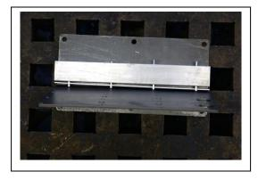
Next you will attach the right side plate using 4each ¼-20x21/2 bolts with washers. In the photo you will notice the shim plate between the right plate and the baseplate block.
