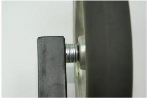
NOTE: Economy contact wheels do not have a spacer between the two bearings. This means if you overtighten the  $\frac{1}{2}$  bolt you will destroy the bearings in short order. Premium contact wheels have a floating spacer between the two bearings and overtightening is not possible.
